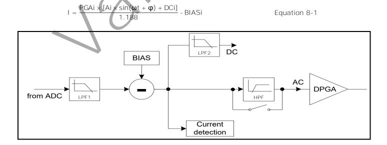
Figure 8-2 Signal Processing for Current Detection
