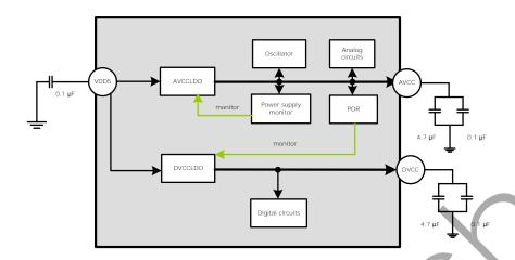
**Figure 4-1 Power Supply Architecture**
