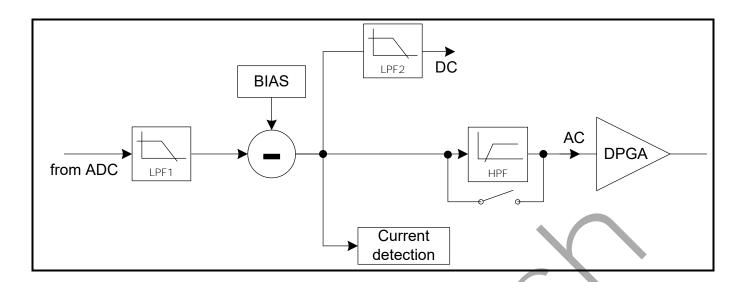
Figure 7-5 Digital Input and DC Removement (Current Signal is Taken as an Example.)
