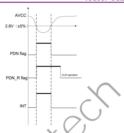
Figure 4-2 Power-Down Interrupt
