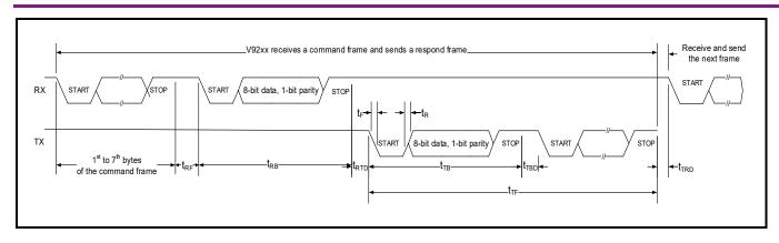
Figure 6-3 Timing of UART Communication
