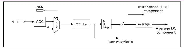
Figure 10-15 Signal Processing in M Channel
