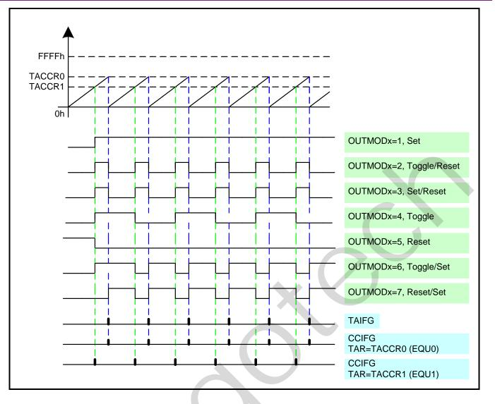
Figure 12-4 Output on Pin TA1 in Up Mode
