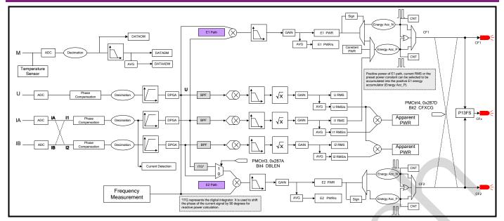
Figure 10-1 Digital Signal Processing in Vango Metering Architecture
