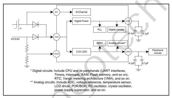
Figure 8-1 Power Supply Architecture
