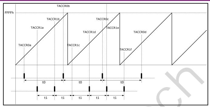
Figure 12-3 Configuring Output Frequency in Continuous Mode
