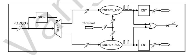
Figure 10-12 Energy Accumulation and CF Pulse Output
