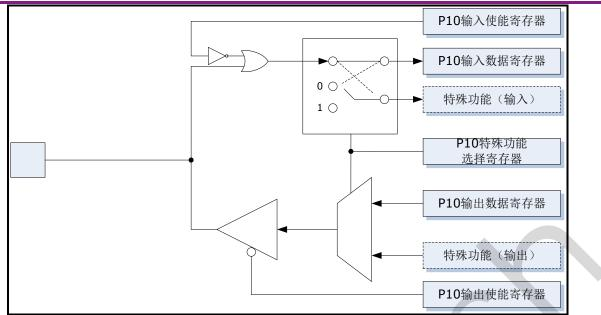
Figure 15-12 Architecture of Each Port of Group P10
