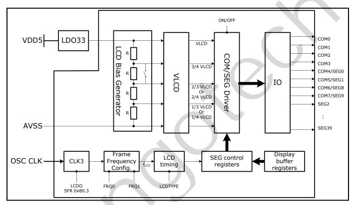
Figure 14-1 LCD Driver Block Diagram
