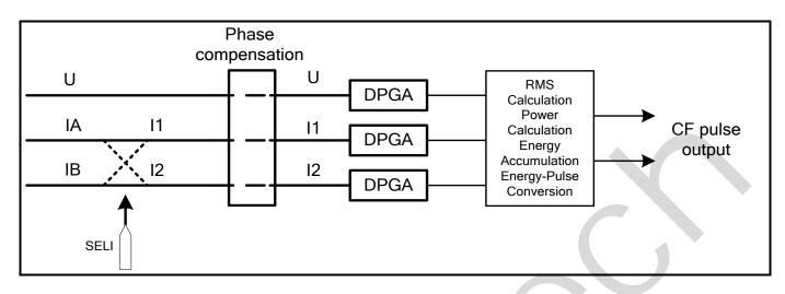
Figure 10-6 Exchange of Current Channels
