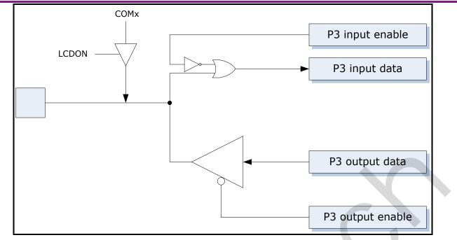
Figure 15-5 Architecture of Each Port of Group P3
