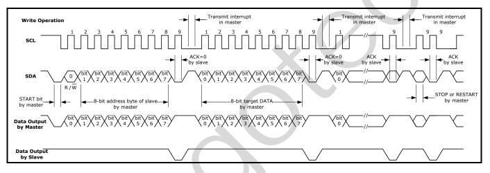
Figure 13-4 Write Operation
