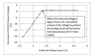
Figure 8-2 LDO33 Output and 5V Power Input
