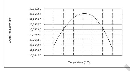
Figure 17-3 Crystal Frequency-Temperature Curve
