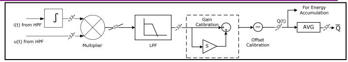
Figure 10-11 Signal Processing for Reactive Power Calculation and Calibration
