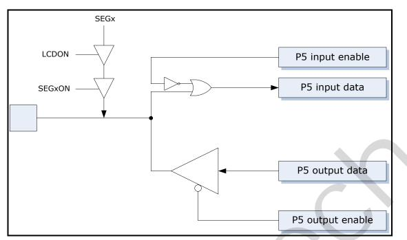
Figure 15-7 Architecture of Each Port of Group P5
