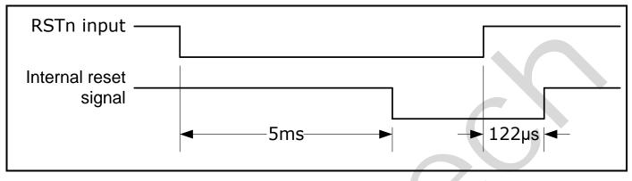
Figure 5-2 RSTn Pin Reset Timing
